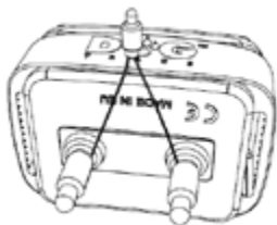
Picture showing test lamp attachment
